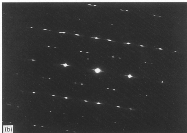
Figure 3 Intradendritic L1 0 martensite in Ni-24 at % Al-21 at % Cr aged for 140 h at 850 °C. (a) Bright-field micrograph; (b) selected-area diffraction pattern ( B = [110] L1 0 ).
